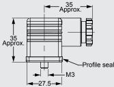
Male electrical connector 3p+PE EN 175301-803 (DIN 43650)
